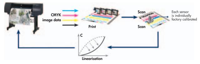
Closed loop colour calibration produces excellent colour consistency, printer to printer, print to print
