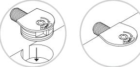
Push twenty HIDDEN CAMS (1F) into the ENDS (A and B), UPRIGHT (C), BOTTOM (F), and SHELF (G). Then, insert the metal end of a CAM DOWEL (2F) into each HIDDEN CAM, except the short edges of the ENDS (A and B).
