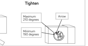
Fasten the UPRIGHTS (C and D) to the TOP (E2). Tighten four HIDDEN CAMS.
