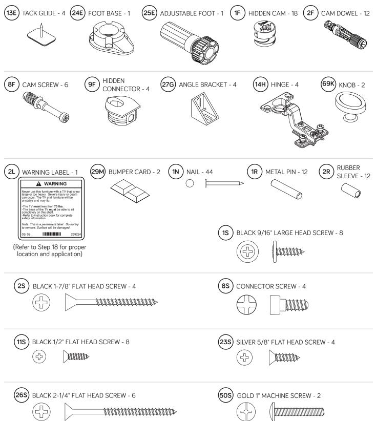
Insert a CONNECTOR SCREW (8S) into each HIDDEN CONNECTOR (9F).
