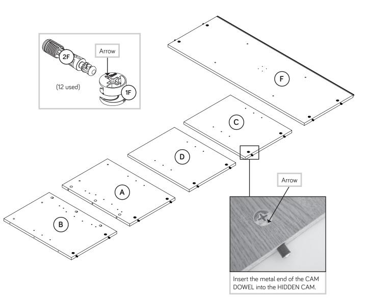
Push six HIDDEN CAMS (1F) into the ENDS (A and B).
