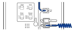
Check that the dialling Mode switch on the underside of the base is set to TB for tone dialling with timed break recall.
