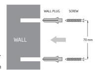
4. Slot the holes on the back of the base over the screw heads and gently pull the phone down to fix it securely in place.
