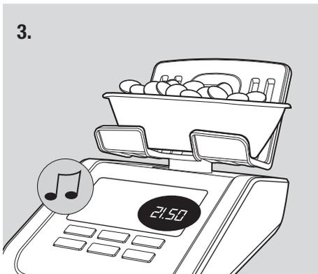
The quantity and value of the coins will be displayed. When the device has finished the count, a 'beep' will sound.
