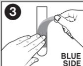
Remove **BLUE** Liner and apply hook to strip. Make sure tab is accessible for future removal.
