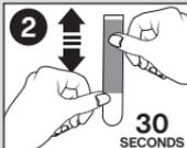
Remove **BLACK** "Wall side" Liner and apply strip to desired location. **PRESS FIRMLY** along the entire strip for 30 seconds.
