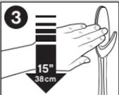
**STRETCH STRAIGHT DOWN ALONG WALL AT LEAST 15 INCHES** (38 cm) until strip releases from wall.
