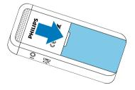
2 Insert the batteries or rechargeable batteries into the device as shown. Make sure the polarity is correct.
