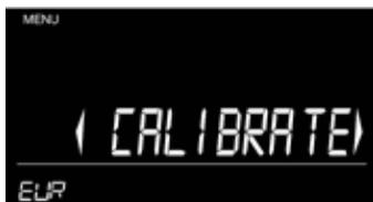
2. The machine will start with the smallest item of coins (e.g. € 0.01). Select the item: Voucher with the [ITEM] button and press [OK] to start the calibration.
