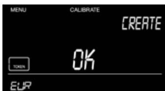
3. Enter the value of the token with the numeric buttons. (e.g. 1.25) and press [OK].
