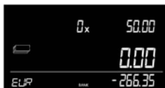
3. Press [OK] to confirm the entry, or press [CE] to clear the entry and re-enter a BANK value. The 6185 will return to count mode. On the screen the BANK icon is displayed, indicating the Bank function is now active - the bank value will be deducted from the total counted amount.
