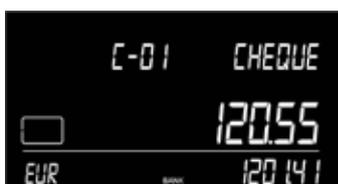
4. Press [OK] to confirm the value. The device stores the counting results and switches to next cheque item (C-02).
