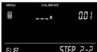
6. Fill in the quantity of a full € 0.01 coin roll with the numeric buttons (example: 50).
