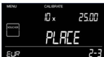
5. Press [OK] to save the settings. The machine will proceed with the next voucher to be calibrated.
