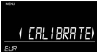
2. Press [OK] to confirm the calibration function. Select the money package you would like to calibrate with the [ITEM] & [◀] [▶] buttons and press [OK].
