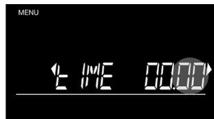
The MINUTES now start blinking. **Short press** **[Left]** **[Right]** to go 1 minute up or down or **long press** to run through the minutes. Press **[OK]** to confirm.
