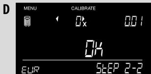
Remove the coin rolls to go to the next calibration step.
