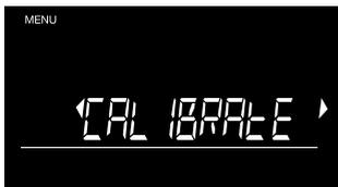
The Safescan 6165 is also able to count coin rolls, banknote bundles and a second coin cup. These first have to be calibrated on the 6165. To enter the calibration mode, press **OK** when the **CALIBRATE** screen is shown. When in calibration mode, use the **←** **→** buttons to navigate to the desired denomination. If you want to switch to the next calibration item, press **MENU**. The sequence is Coin Rolls - Banknote Bundles - Coin Cup.
