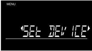
When the **SET DEVICE** screen is shown, you can change several device settings. Press **[OK]** to enter this menu item. When in the SET DEVICE mode, use the **[Left]** **[Right]** buttons to navigate through the sub-items.
