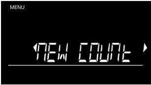
When you want to start a new count and erase all existing results, press **[OK]** when the **NEW COUNT** screen is shown.
