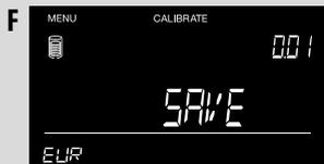
Press to save. The roll has now been calibrated and is saved in the machine.
