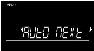
To activate or de-activate the function, press
