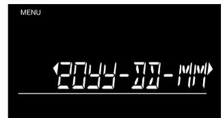
Navigate through the date formats by using **[Left]** **[Right]**. Press **[OK]** to confirm the desired format. Now set year, month and day in the same way.
