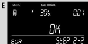
Select the number of coins that the rolls will contain by using the buttons and press .
