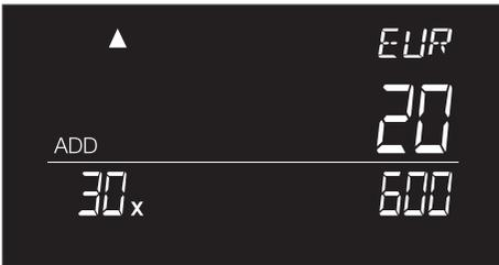
**6. ADD mode:** The device will add the value and also show the total quantity of all scanned banknotes on the display.
