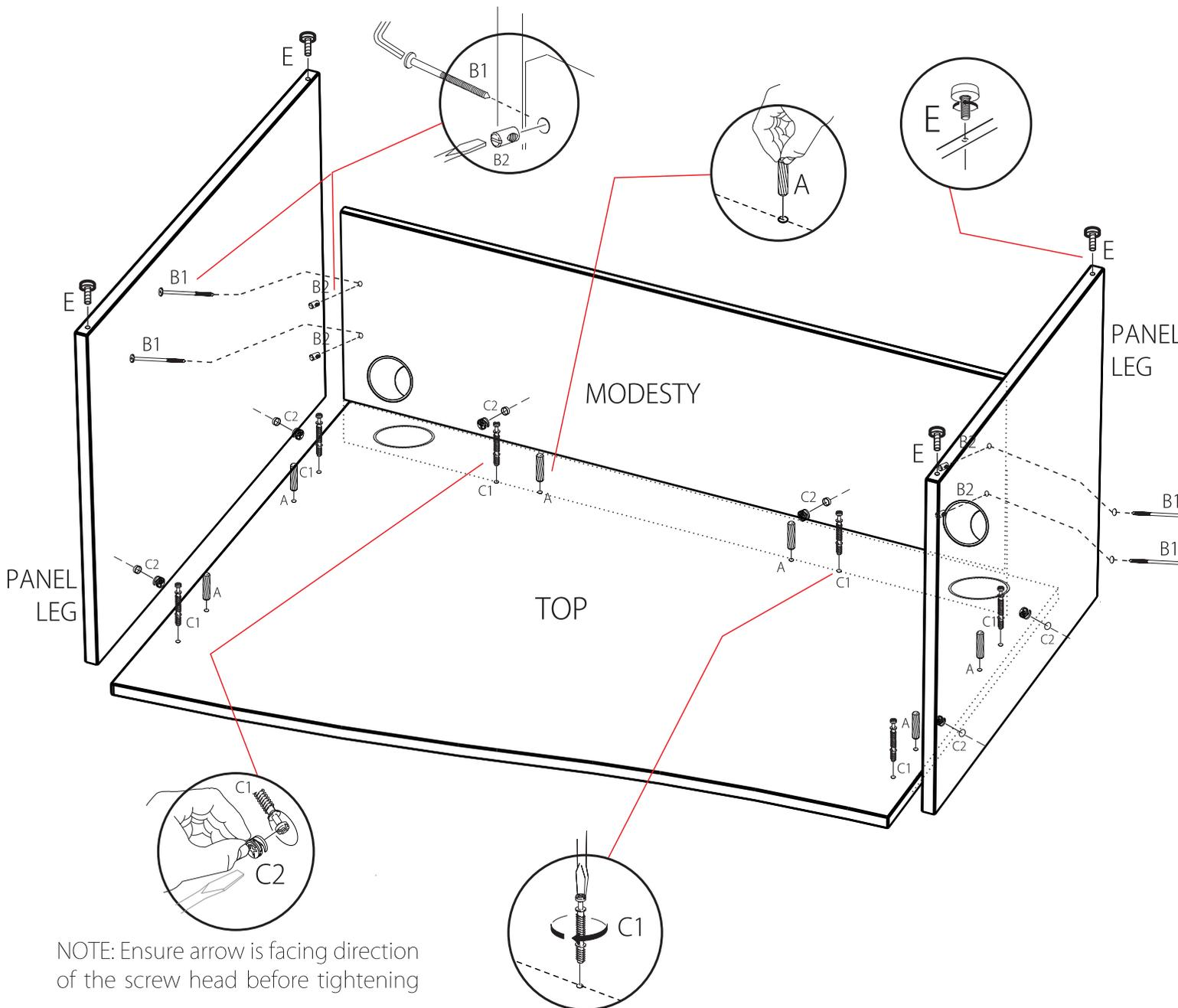
NOTE: Ensure arrow is facing direction of the screw head before tightening
