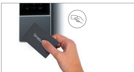
Clocking with RFID proximity card or PIN code
