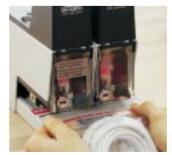
Two R105E staplers mounted inline. Slim design enables staples to be placed close together.
