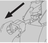
5050e is extremely durable. Every time you replace the cassette, you automatically replace the driver blade and staple former blade. This unique, patented feature enables you to staple up to 50 sheets of 80gsm paper at a time at least 500,000 times.
