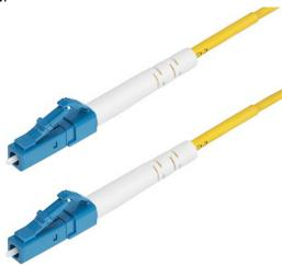
OS2 LC to LC Single Mode Simplex Fiber Optic Patch cable facilitates connectivity across 40G/100G networks. It supports Coarse Wavelength Division Multiplexing (CWDM) across an extended wavelength range of 1260-1625nm, improving channel isolation for optimal signal strength over long distances.
