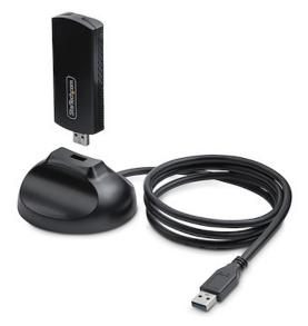
This USB Wi-Fi 6E Network Adapter connects to desktop or laptop computer enhancing its capabilities and enables high-speed and low-latency wireless communication in the 6GHz band with combined tri-band speeds of up to 5400 Mbps.
