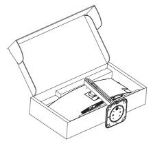
While keeping the release button pressed, tilt the base and slide it out.
