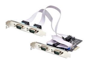
Add serial communication support to a desktop computer or Small Form Factor (SFF) system, using this 4-Port Serial PCI Express Card. The four DB9 ports can be independently configured to support RS-232, RS-422, and 2/4-wire RS-485 standards, for communication with compliant serial peripheral devices.
