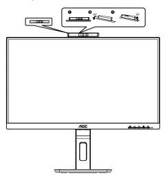
Noted: Turn the lens down 90° to block the lens. The microphone can be turned off using the video software or the MIC OFF shortcut key.
