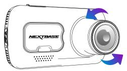
Gently rotate the front bezel to adjust the filter. Rotate the filter until the windscreen reflection can no longer be seen on the Dash Cam display (see below).
