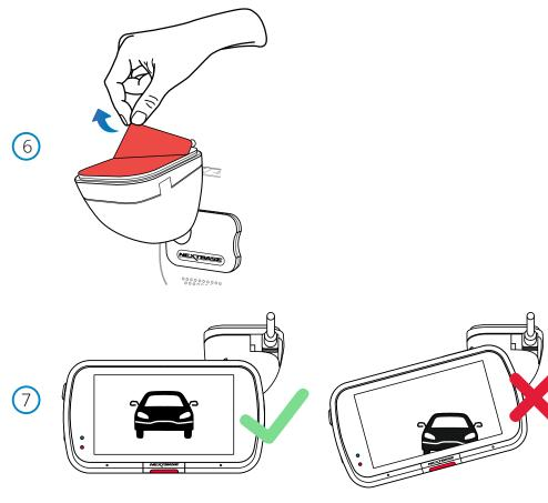
6 Remove the adhesive cover layer Peel back the red cover layer to expose the adhesive surface, ready to mount on your windscreen.
