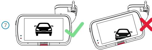
7 Straighten the Dash Cam Ensure that the Dash Cam is horizontal and faces straight out of the windscreen. Ensure that objects on the Dash Cam display appear level, and adjust as required.
