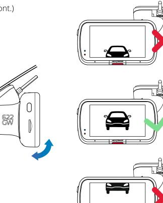
9 Adjusting the Dash Cam With the mount attached to the windscreen, ensure that objects on the Dash Cam display are level and adjust as required. Ensure that the road ahead is at the centre of the image, in the central third of the display. If too much of the sky is visible it may risk underexposing details on the road; ensure that the road ahead is clearly visible on the Dash Cam display. Do NOT attempt to adjust the Dash Cam while driving.
