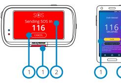
During countdowns the screen on the Dash Cam will alternate between red and black backgrounds to be as noticeable as possible.
