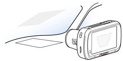
Do not place fingers on the glass lens of the filter. Do not adjust the filter while in control of the vehicle
