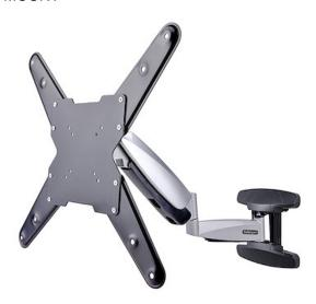
The steel and aluminum construction of this VESA TV Wall Mount supports TVs from 23" to 55" and up to 66lb (30kg). The arm assembly provides smooth one-touch height adjustment thanks to its spring-loaded mechanism that acts as a counterbalance. The VESA plate supports mounting patterns of 75x75 to 400x400.
