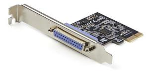
This PCIe Parallel controller card installs into an available PCI-Express x1 slot in your computer and enables you to add DB25 parallel communication port to your system.
