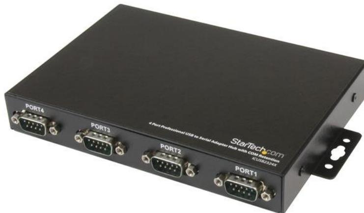
The ICUSB2324X 4 Port Professional Grade USB Serial Adapter converts a single USB port to four RS232 serial ports allowing you to connect to, monitor and control your serial devices. Rugged metal construction and sturdy wall-mount brackets provide a robust solution for both harsh industrial environments and simple desktop installations.
