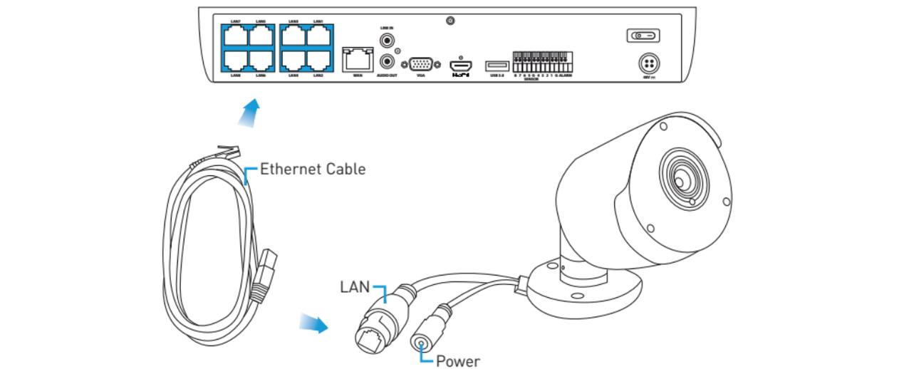
**Please note:** The power connector is provided as an alternative power option if required. Your NVR will provide power over the Ethernet cable when connected and a separate power adapter is not required.
