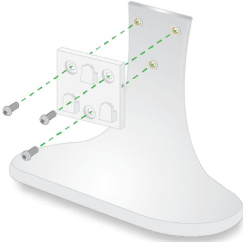
2. Slide the Orbi satellite onto the wall-mount bracket.
