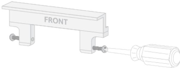
2. Place the lock on top of the wall-mount bracket.
