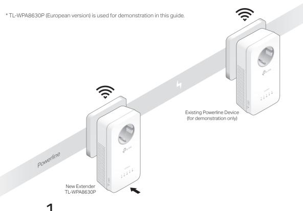
Plug in the new extender near one of your existing powerline devices.
