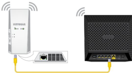
1. Set the **Access Point/Extender** switch to **Access Point**
