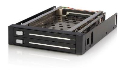
This 3.5in SATA hard drive hot-swap bay allows you to install two 2.5in SATA hard drives (HDD) or solid state drives (SSD) in an available/unused 3.5in floppy drive bay.
