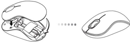
4. Replace the battery cover, carefully fit the cover until it clicks into place.
