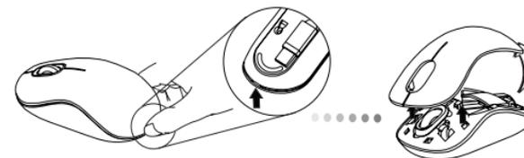
2. Remove the battery safety clip by squeezing the center of the clip and sliding it back, towards the rear of the mouse. Lift up and rotate the clip out of the way.
