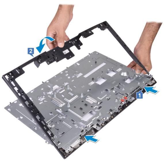
2 Replace the 15 screws (M3x5) that secure the middle frame to the display assembly base [2].
