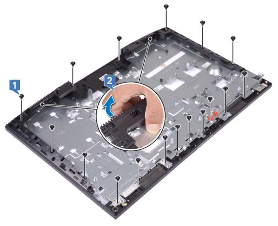
5 Lift the middle frame off the display assembly base [1].
