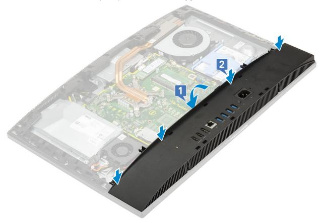
3 Replace the four screws (M3) that secure the base cover to the display assembly base.
