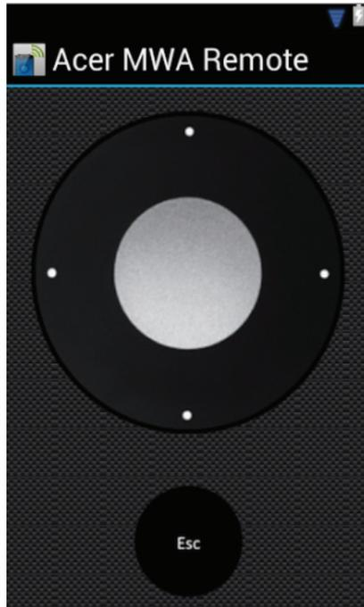
4. Use the left, right, up, down, or select (center) keys to control the MWA2 Wireless Adapter. the **Esc** key acts as a back button.
