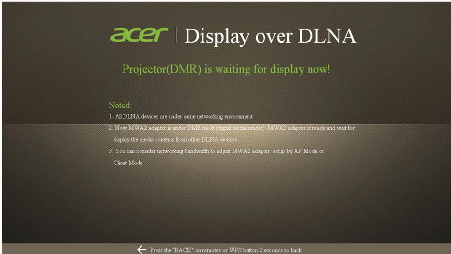
1. **On the projector/monitor/TV**, go to the **DLNA** screen by using that device's remote control, or by briefly pressing the WPS button twice on the MWA2.
