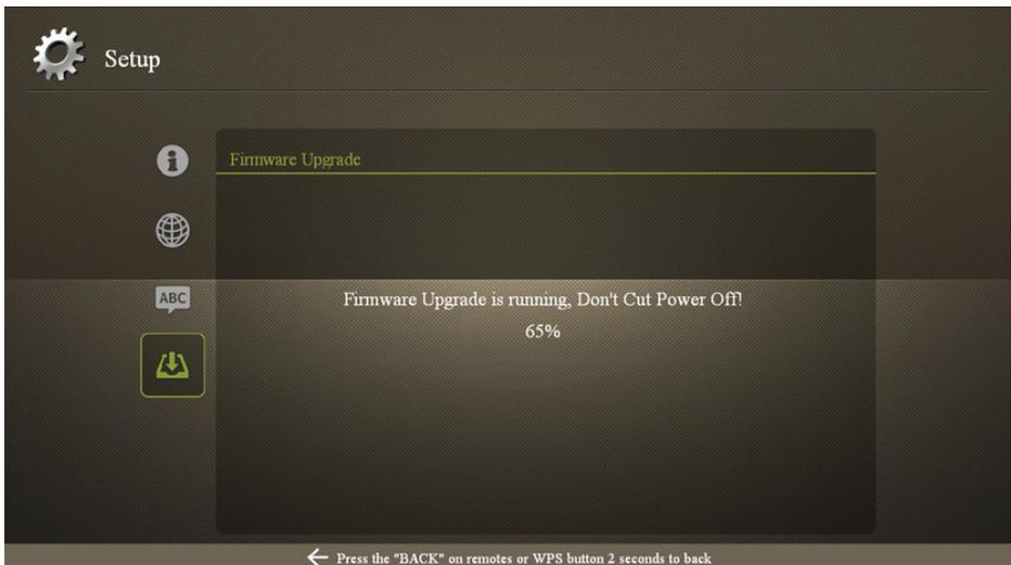
**Caution:** Do not turn off the device or unplug the MWA Wireless Adapter at any time during the firmware upgrade.
