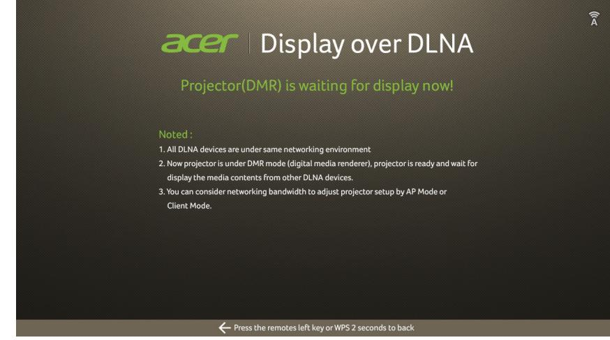
1. On the projector/ monitor/ TV, go to the DLNA screen by using that device's remote control, or by briefly pressing the WPS button twice on the MWA2.
