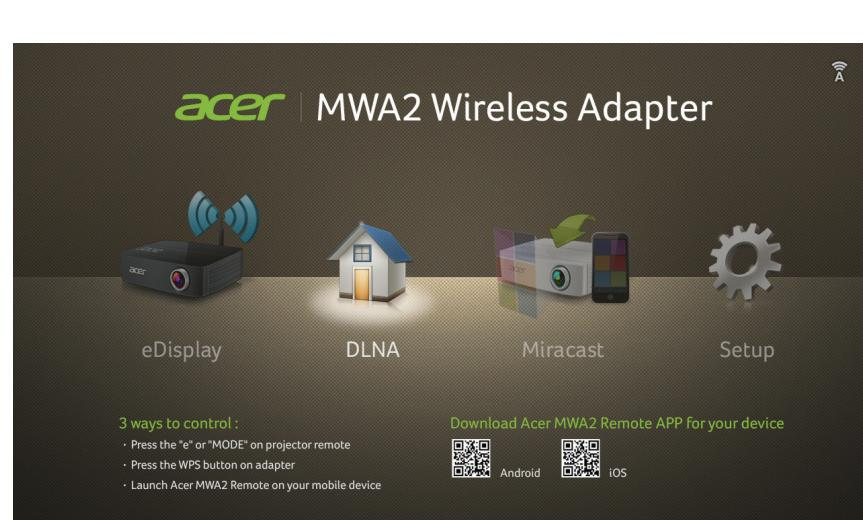
There are several ways to choose between the different connections (eDisplay, DLNA, or Miracast), either by using the projector/ monitor/ TV's remote control (RCP), by pressing the WPS button on the Wireless Adapter, or by selecting on the mobile device itself.
