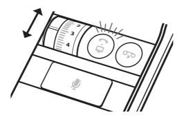
**6.6** Press the Mute button to mute the headset microphone. The Mute indicator will be ON. To un-mute the headset microphone, press the Mute button again. The Mute indicator will go OFF.
