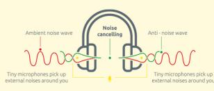
Headphones with active noise canceling are headphones that reduce unwanted ambient noise. This differs from passive headphones, which, when they reduce ambient noise at all, use techniques such as sound isolation.
