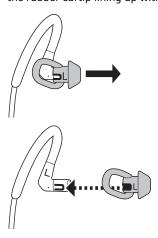
**Clean the eartip** When needed, clean the eartip with an alcohol wipe or a cotton swab dipped in isopropyl alcohol.
