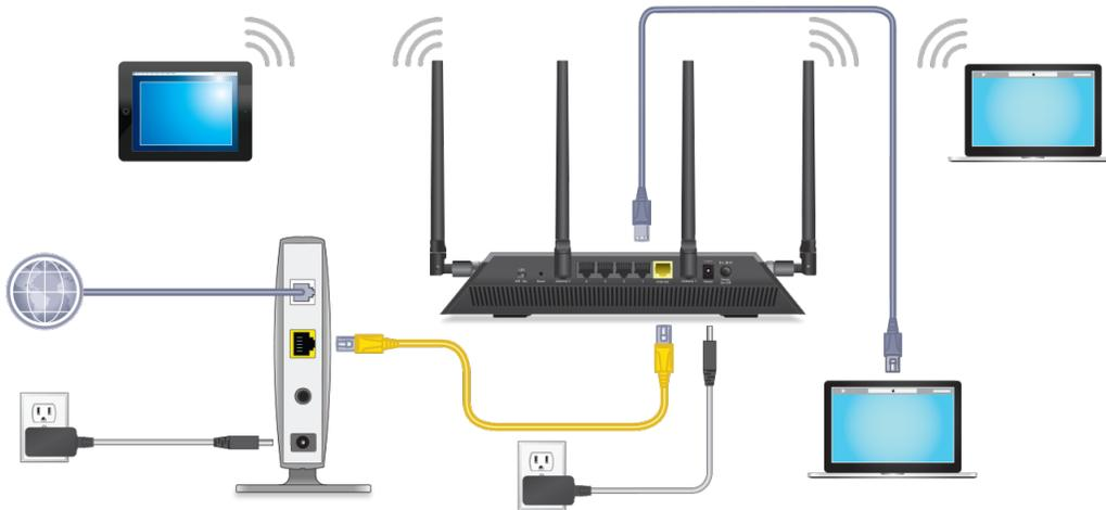
Figure 6. Router cabling
