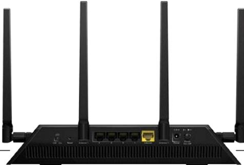
eSATA port | LED On/Off | Gigabit Ethernet | Internet | USB 3.0 ports
