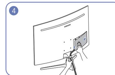
Grab the stand with one hand and use the thumb on your other hand to remove the COVER-CLEAN BACK TERMINAL in the direction of the arrow.
