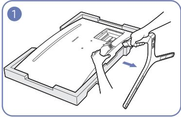
Place the protective Styrofoam (cushion) included in the package on the floor and place the product facing down on the Styrofoam, as shown in the image. If Styrofoam is unavailable, use a thick sitting mat. While holding the monitor with one hand, pull the stand neck with your other hand to detach the stand as shown in the figure.
