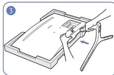
Place the protective Styrofoam (cushion) included in the package on the floor and place the product facing down on the Styrofoam, as shown in the image. If Styrofoam is unavailable, use a thick sitting mat. Hold the back of the monitor as shown in the figure. Push the assembled stand into the main body in the direction of the arrow as shown in the figure.
