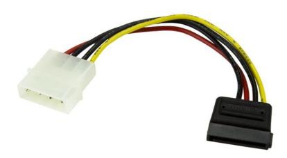
This 6in 4 Pin (LP4) Molex to SATA power adapter cable features one 4 Pin Molex (LP4) male connector and one female SATA power connector, allowing you to power a Serial ATA hard drive from a conventional LP4 connection, eliminating the need to upgrade the computer power supply for compatibility with the SATA hard drive.
