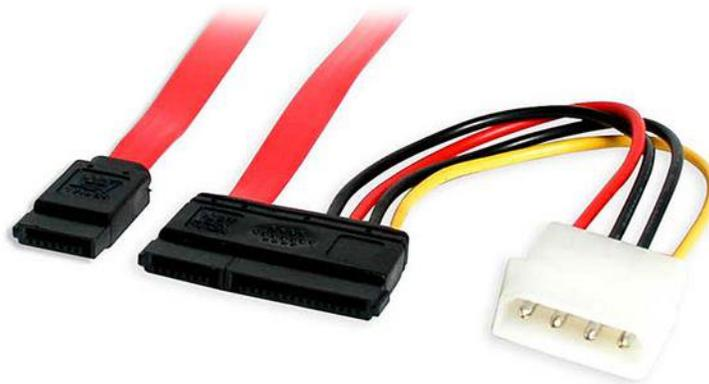
The SATA18POW SATA Data and Power Cable features a combination 22-pin SATA receptacle data and power connector as well as an Molex (LP4) power connector and SATA receptacle data connector, allowing you to create a conventional Serial ATA data connection to a computer while powering the drive through an LP4 connection to the computer power supply.
