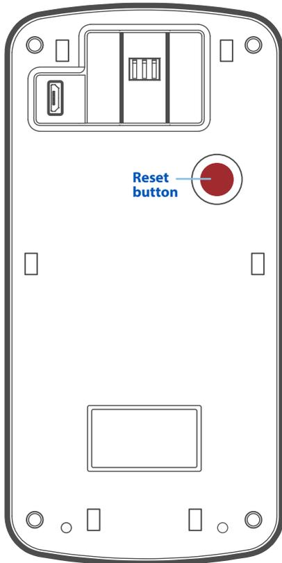
Press the **Reset** button for two seconds.
