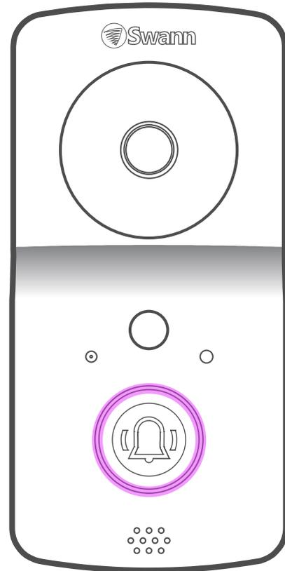
The light ring on the Doorbell glows purple and turns off when the Doorbell has restarted. It can take about 30 seconds for the Doorbell to restart.
