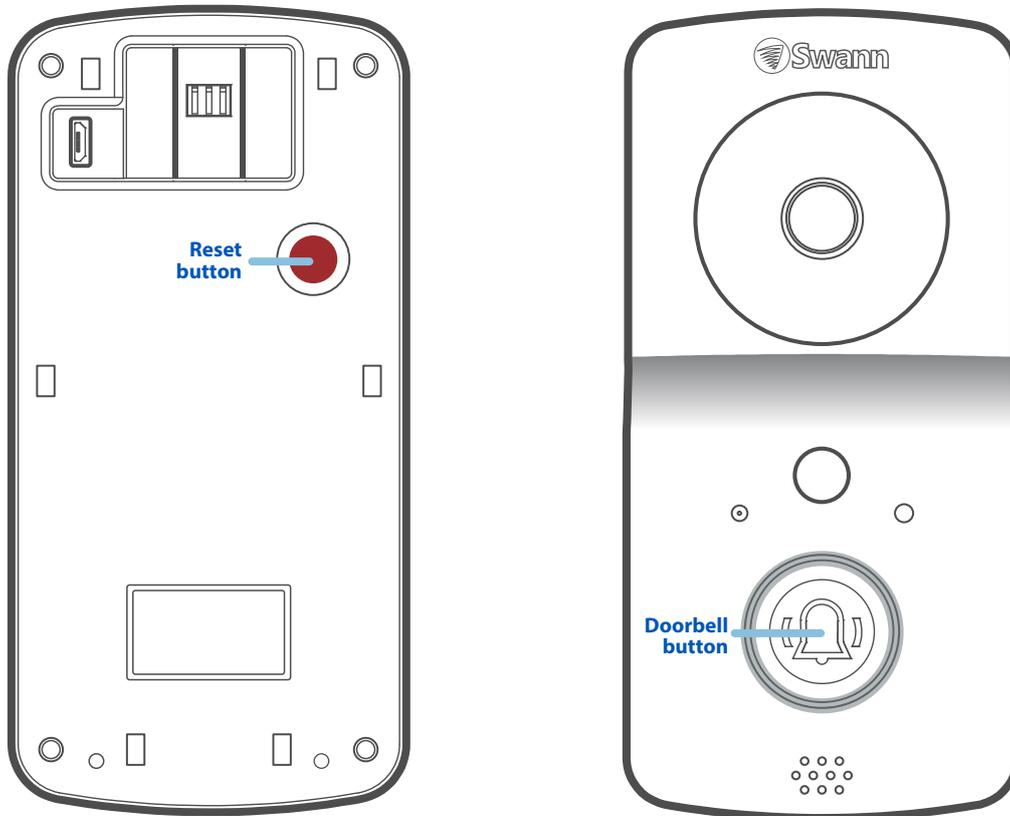
Press and hold the **Reset** and **Doorbell** buttons at the same time, then release the **Reset** button and continue holding the **Doorbell** button for another 15 seconds. The LED ring will blink purple once, then blue before turning off after you release the Doorbell button.
