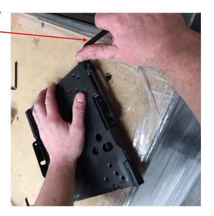
Pull back the top plate and release the lever once this is at the furthest back position to reveal the four fixing locations.
