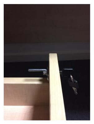
The below image shows the mechanism in the unlocked position. If this mechanism is in the unlocked position when you close the drawers then the key will turn and you will be able to lock the drawers.
