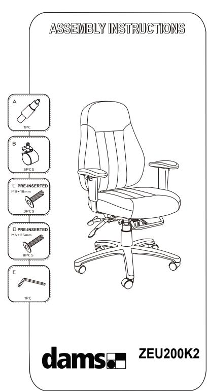
Do not tighten bolts fully until you have completed assembly. Please note the fixing screws are located in their fixing points if not found in the parts bag. Should you require any assistance in assembling your goods please contact customer services on 0151 548 7111 between 9am/4:30pm.
