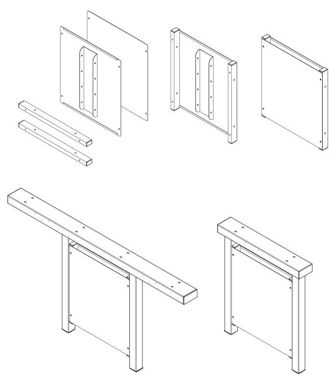
Can be used with both 1600mm and 800mm intermediate leg frames.
