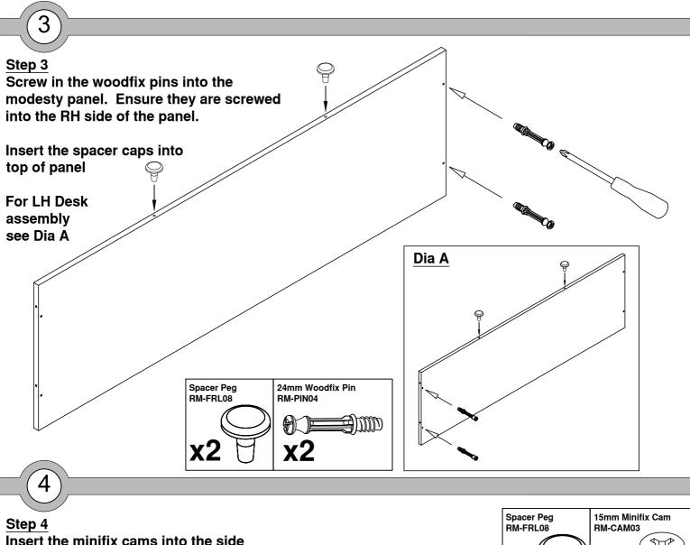
Insert the minifix cams into the side panel. Ensure they are inserted into the LH side of the panel and that the fitting is pushed all the way down and the arrow guideline is aligned with the hole in the edge of the panel.
