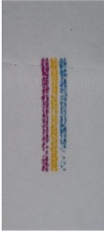
Fig. 26: Color sample released by automatic print head cleaning
