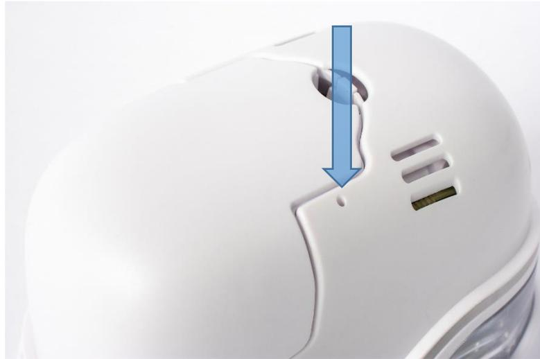
Fig. 52: Opening for device reset
