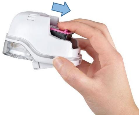
Fig. 45: Pull out ink cartridge
