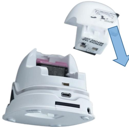
Fig. 10: Battery contact insulating tape
