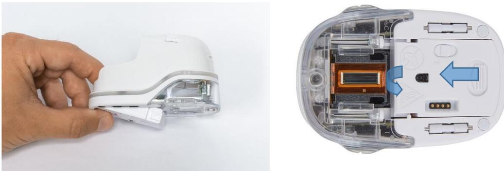
Fig. 11: Opening the sliding panel
