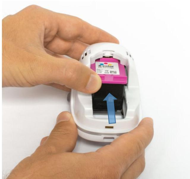
Fig. 13: Insert ink cartridge
