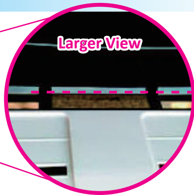
Close the cover, and pull out the film for about 30cm.
