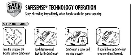
area more than 3 seconds shredder will shut off
